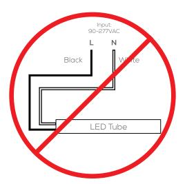
CAUTION: Do NOT attempt to connect both the Load (Black Wire) and the Neutral (White Wire) to the same side of the LED Tube. Doing so will damage the tube and void the warranty.
